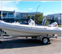
The Smuggler Strata 490 RIB is unrivalled in performance and quality. This boat has a 23 degree deep vee hull so the ride is comfortable and safe, no matter what the conditions. The Strata 490 comes standard on a trailer with a range of console options to suit your needs. It can also be used as a tender, with lifting rings and strops built into the hull. The beauty of this RIB is the ability to custom finish your console options, and to be used on a trailer or as a tender.
