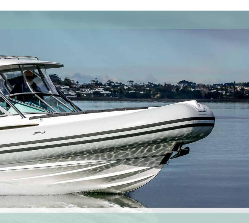
ike all of Smuggler's proven Strata range of RIBs, the 780SS is a combination of fibreglass hulls and Hypalon tubes and these make for a spacious, stable platform in a range of configurations.
