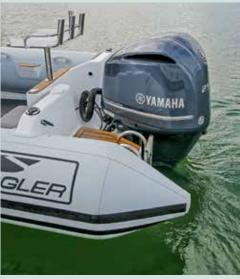
is slightly over the standard road-legal towing width. An overwidth board is provided for daytime towing, while the tubes can also be partially deflated to reduce the external beam sufficiently to allow the boat to be towed at night.
